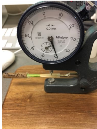
Spine measured at .49mm.
