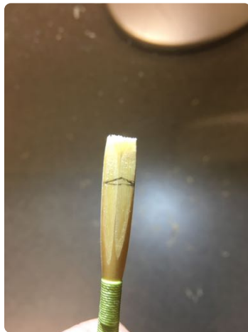
Blank with drawn tip definition.
