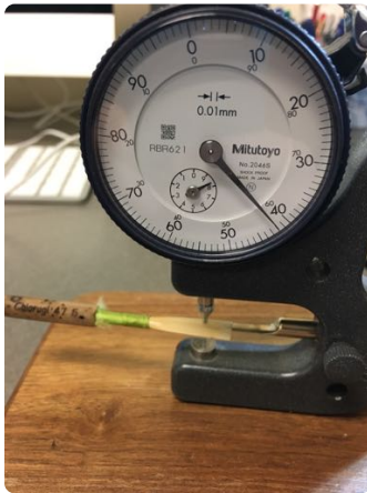
Channel measured at .42mm.
